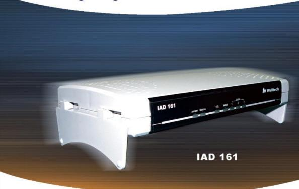
The IAD 161 is a one-port telephone extension and three ports SOHO Router to IP network gateway. It provides Data transfer by 10/100Mbps, telephone services and T.38 fax over IP network with easily operation and configuration. It is most suitable for SOHO and small-to-medium enterprise in Internet communication environment.
